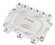
Figure 1: HybridPACK1-DC6 IGBT module.
